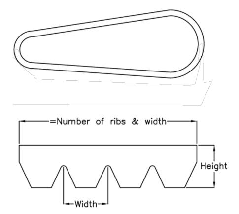
$\begin{array}{ll} \text{Datum Llength} = 2705 \\ \text{Height} &= 9.5 \\ \text{Number of ribs} = 48 \\ \text{Pitch} &= 4.7 \end{array}$
